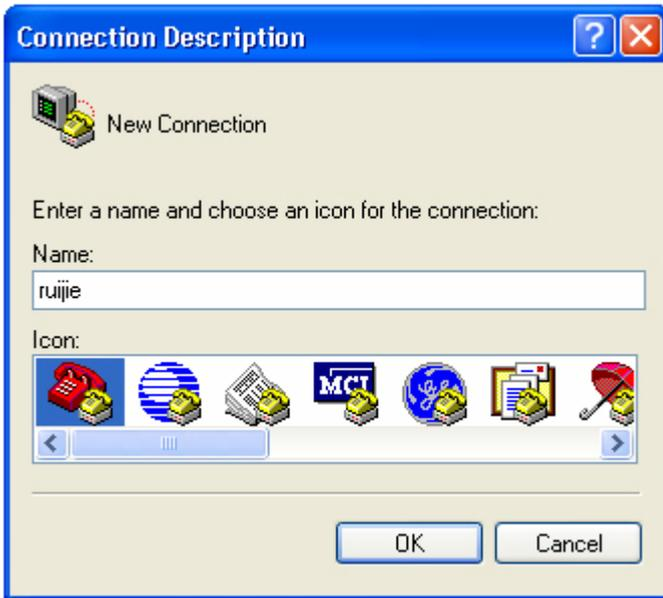
Enter the name of the new connection and click **OK** to display the following page. Choose the series port used currently in the column [use when connecting].
