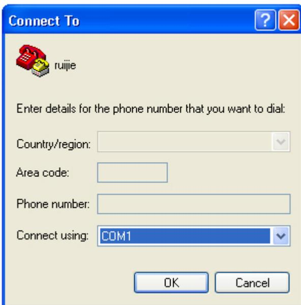
After choosing the series port, click **OK** to display the series port parameter setting page, set the baud rate at 9600, data bit at 8, parity check as none, stop bit at 1 and flow control as none.
