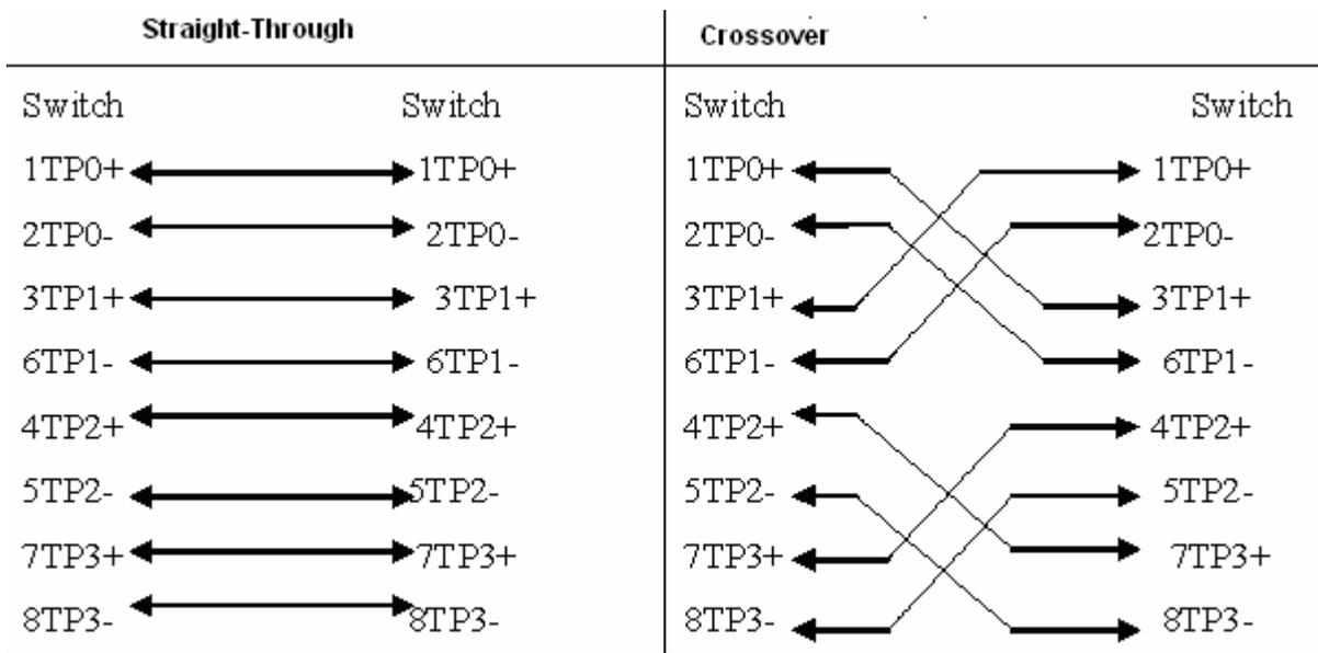
In addition to the above cables, the 100BASE-TX/10BASE-T can also use 100-ohm Category-3, 4, 5 cables for 10 Mbps, and 100-ohm Category-5 cables for 100 Mbps, both of which can be up to 100 m. 0 shows the pinouts of the 100BASE-TX/10BASE-T.
